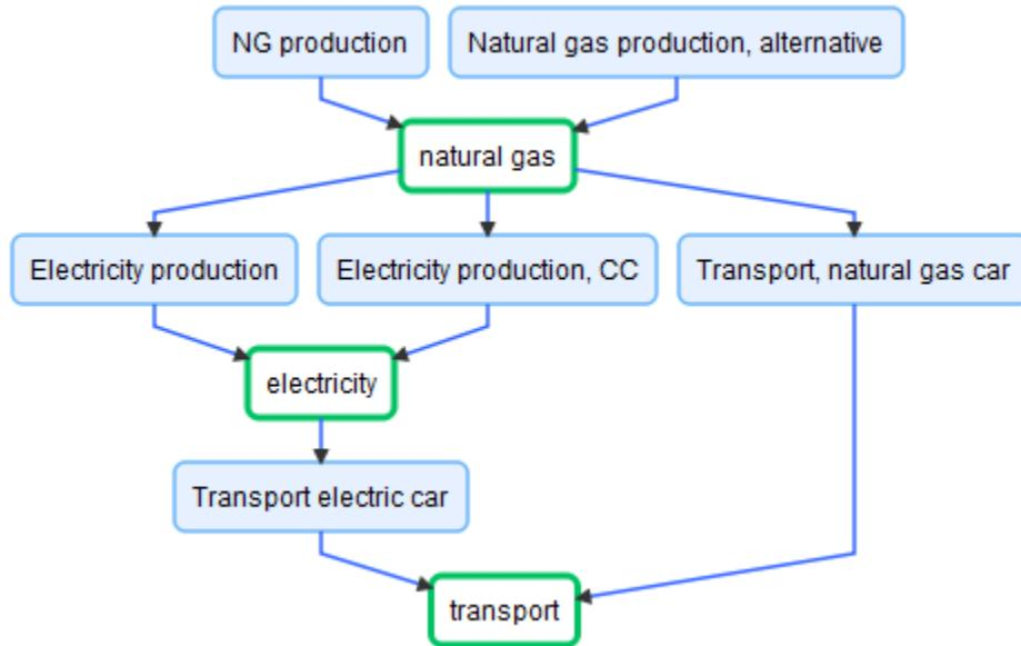
Linked Module Systems are created by combining modules based on their product inputs and outputs. As shown in the example, the product based linking allows to efficiently specify alternative supply chains.
